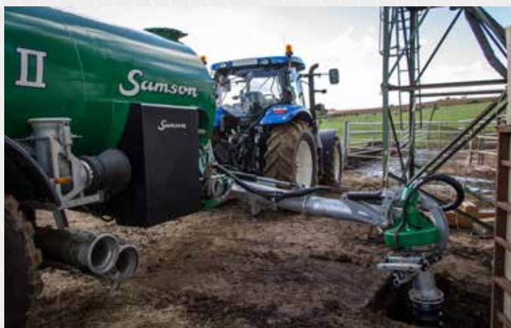
Direct filling from underground storage of slurry
