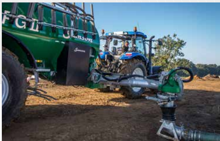
Filling by filling funnel
