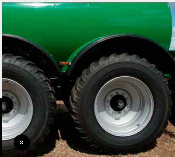
The large wheels reduce rolling resistance.
