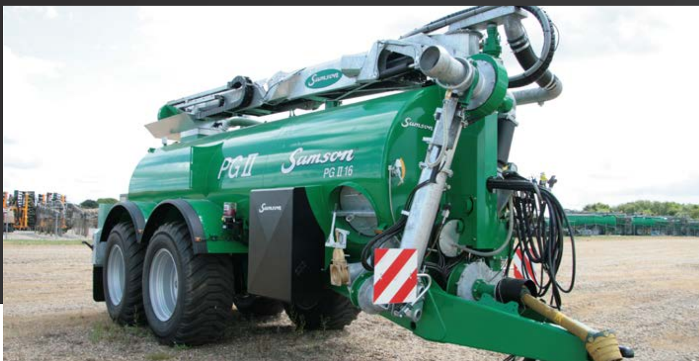
Single-articulated SAP arm (SAP1) with or without pump
