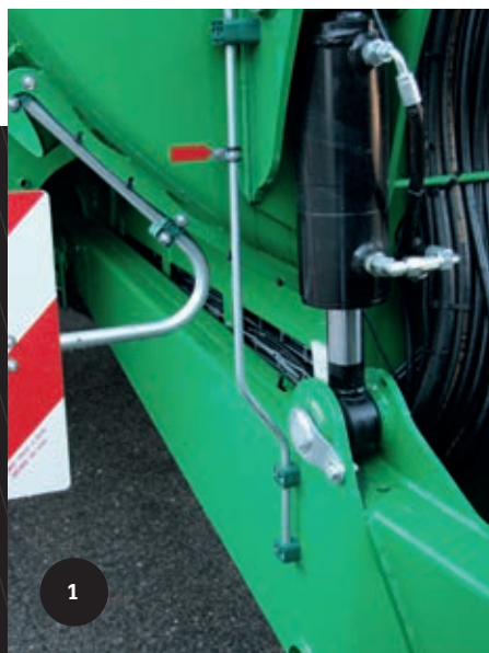
Drawbar suspension gives optimal driving comfort. The height can also be adjusted.
