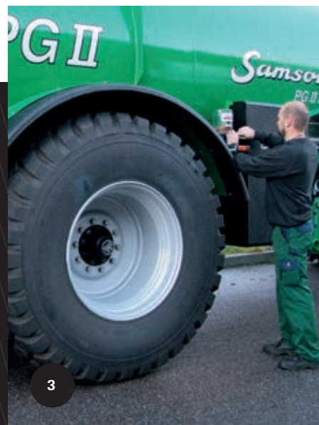
The large wheels reduce rolling resistance.
